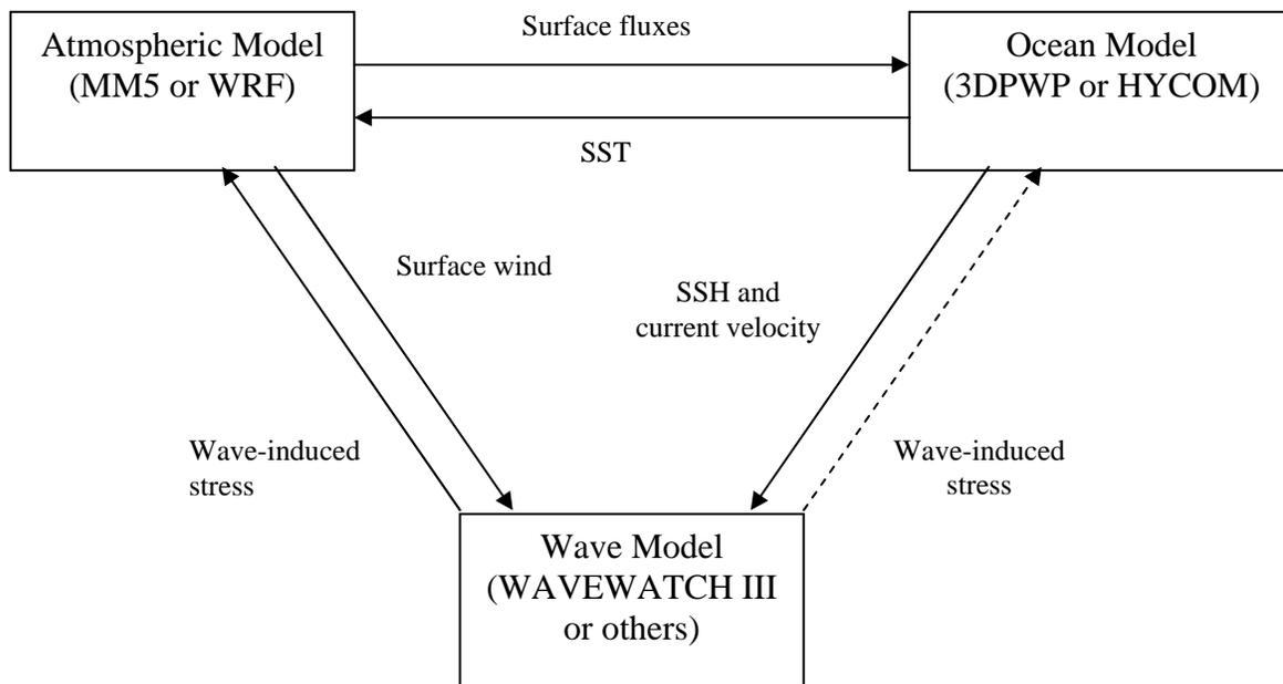
Figure 1. Schematics of a fully coupled atmosphere-wave-ocean modeling system with the component atmosphere, surface wave, and ocean circulation models, as well as the coupling parameters among each of the components.
