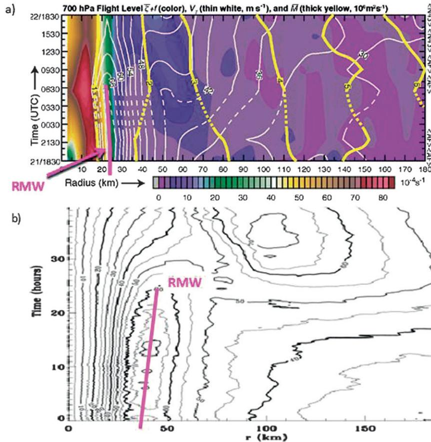
FIG. 1. (a) Azimuthally averaged vorticity (shading;  $10^{-4} \text{ s}^{-1}$ ), tangential wind speed (white lines;  $\text{m s}^{-1}$ ), and absolute angular momentum (yellow lines;  $10^6 \text{ m}^2 \text{ s}^{-1}$ ) at 700 hPa in Hurricane Rita [adapted from Bell et al. (2012)]. (b) Azimuthally averaged tangential wind speed ( $\text{m s}^{-1}$ ) at 2786-m height (adapted from T13). Magenta lines denote the approximate location of the radius of maximum wind.
